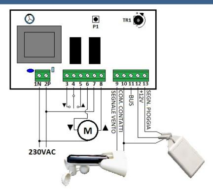
P1 (RESET BUTTON): used to reset the status of ALARM (wind or rain). Press it and keep it pressed until the ALARM status is exited
