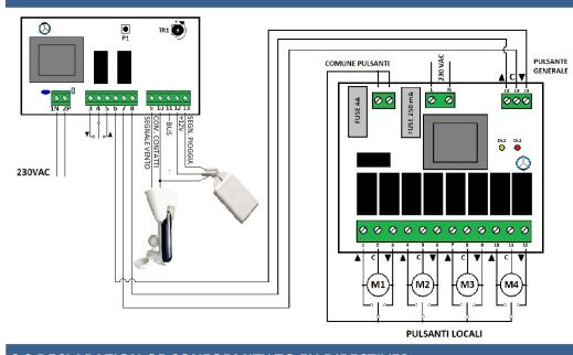
The control unit 703 also allows the possibility to exploit the command output to CLEAN CONTACTS, rather than in voltage (for the management of other control units).
